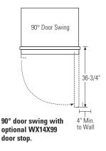
When installing an All-Refrigerator and All-Freezer side-by-side, allow 25" for a full 130° door swing, or 15" min. on the hinge sides for pan access.
